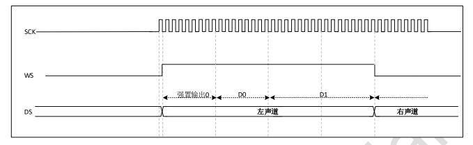
Figure 29-24 I2S LSB justified standard (24-bit frame, CPOL = 0)
