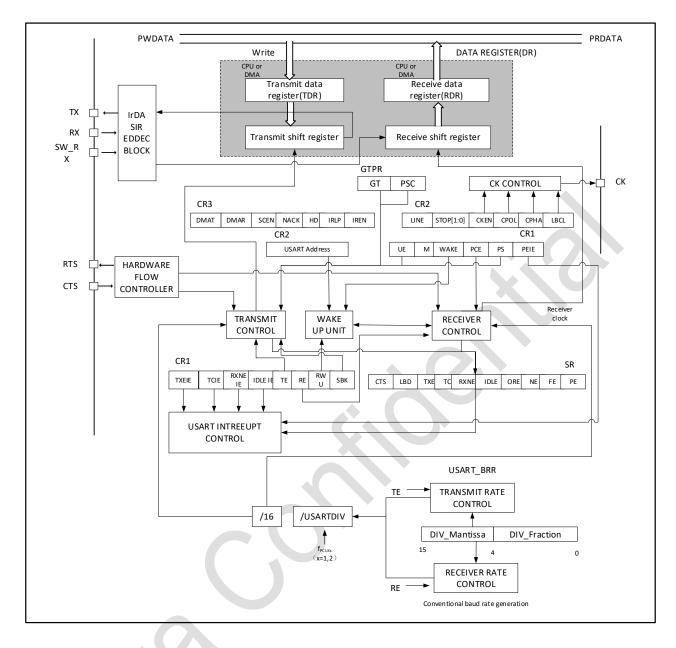
Figure 28-1 USART block diagram
