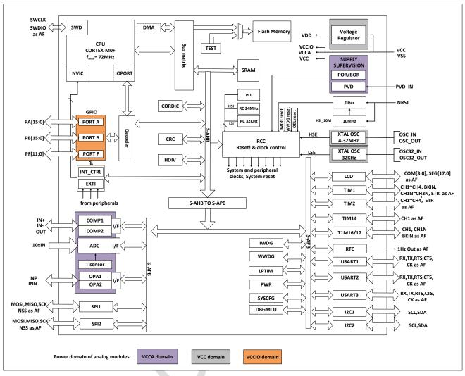
Figure 2-1 System architecture
