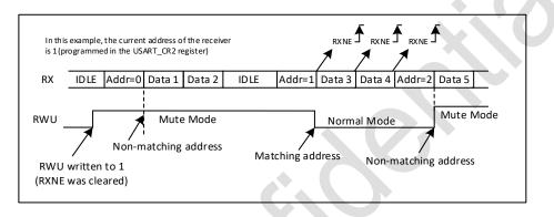
Figure 28-8 Mute mode using address mark detection
