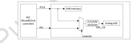
Figure 14-4 ADC clock scheme
