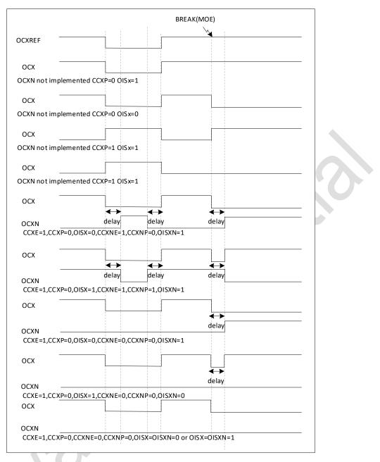
Figure 21-20 Output behavior in response to a break
