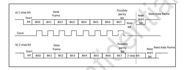
Figure 28-3 Configurable stop bits
