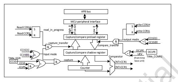
Figure 19-27 Capture/compare channel 1 main circuit
