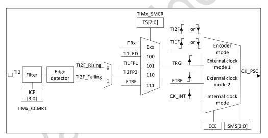
Figure 18-23 TI2 external clock connection example
