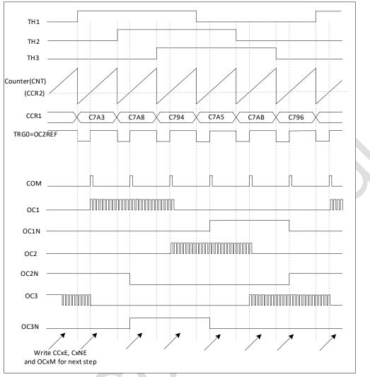
Figure 18-45 Example of Hall sensor interface
