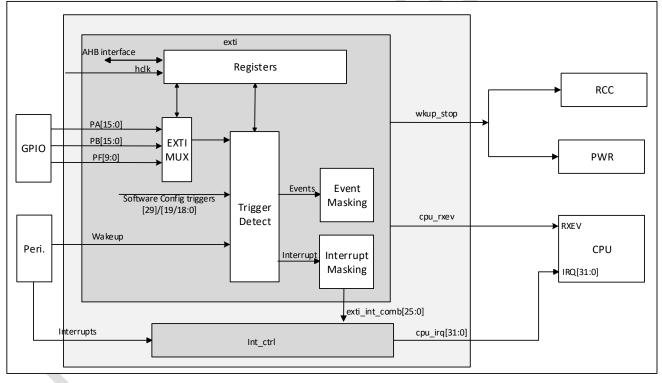
Figure 12-1 EXTI block diagram
