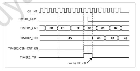
Figure 19-43 Trigger timer 2 with an update of timer 1
