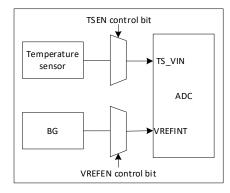
Figure 14-14 Temperature sensor and reference voltage channel
