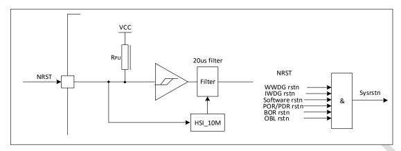
Figure 7-1 Simplified diagram of the reset circuit
