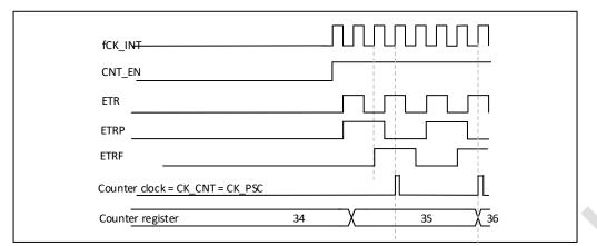
Figure 19-25 Control circuit in external clock mode 2
