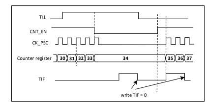
Figure 19-37 Control circuit in Gated mode
