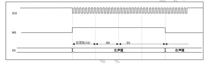
Figure 29-25 I2S LSB justified standard (24-bit frame, CPOL = 1)
