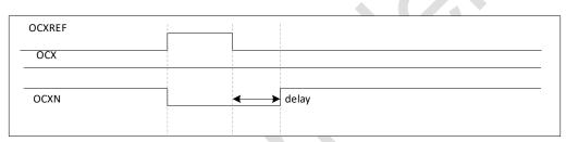
Figure 21-19 Dead-time waveforms with delay greater than the positive pulse.
