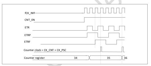
Figure 18-26 Control circuit in external clock mode 2
