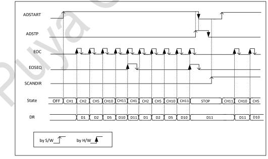
Figure 14-8 Continuous conversion of a sequence, software trigger
