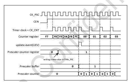
Figure 19-2 Counter timing diagram with prescaler division change from 1 to 2
