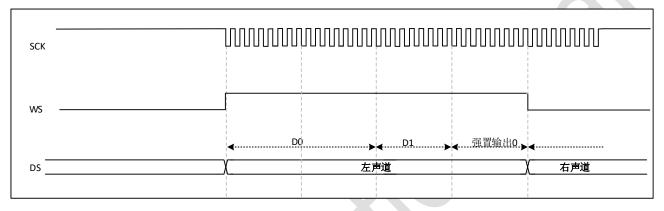
Figure 29-19 I2S MSB justified standard (24-bit frame, CPOL = 1)
