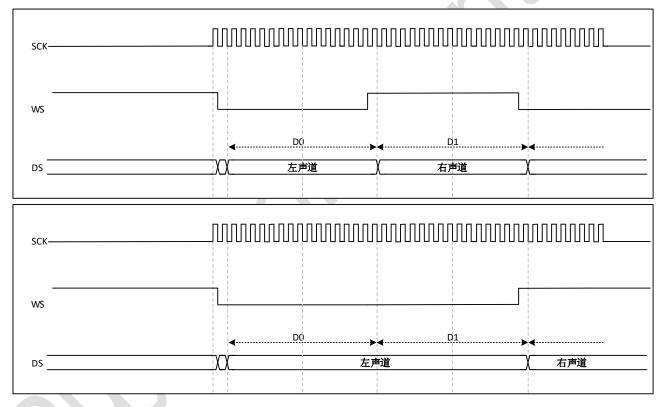
Figure 29-11 I2S Philips protocol (16/32 bit full accuracy, CPOL = 0)
