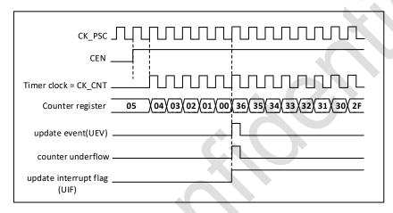
Figure 19-10 Counter timing diagram, internal clock divided by 1
