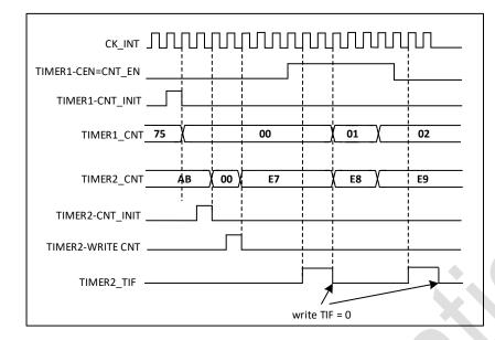
Figure 19-42 Timer 2 can be controlled by enabling Timer 1
