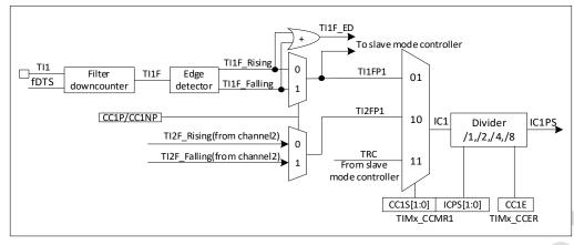
Figure 18-27 Capture/compare channel (example: channel 1 input stage)
