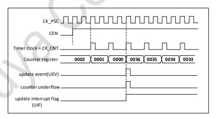
Figure 19-11 Counter timing diagram, internal clock divided by 2
