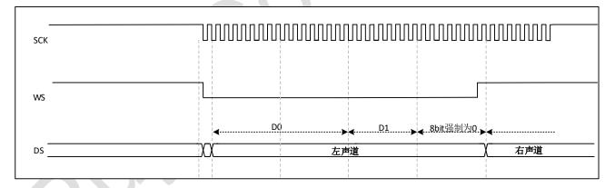
Figure 29-14 I2S Philips protocol (24-bit frame, CPOL = 1)
