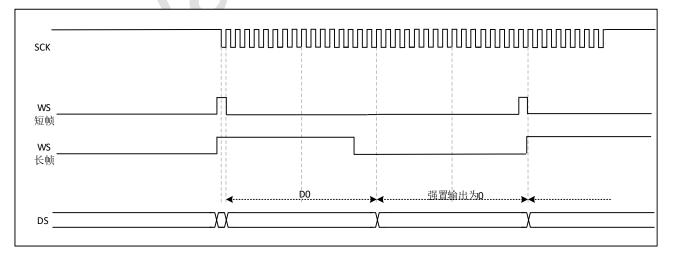
Figure 29-31 I2S PCM standard (16-bit extended to 32-bit, CPOL = 1)
