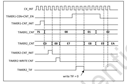
Figure 19-44 Trigger timer 2 with enabling of timer 1
