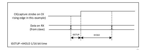
Figure 28-12 RX data sample/hold time
