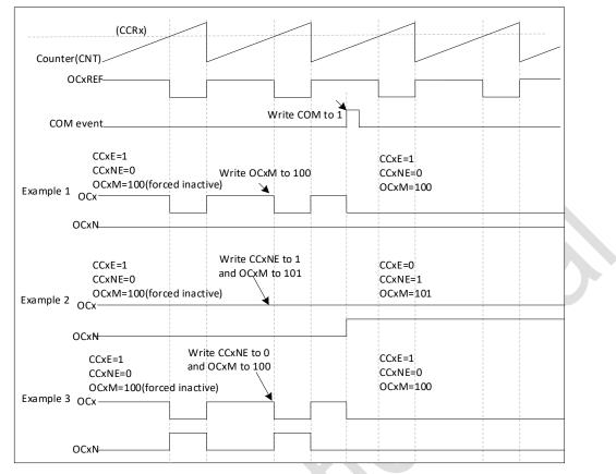
Figure 18-40 6-step generation, COM example (OSSR=1)
