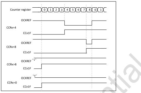
Figure 19-31 edge-aligned PWM waveform (ARR = 8)
