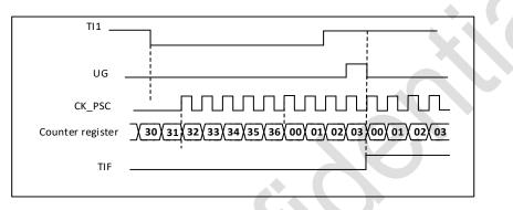
Figure 19-36 Control circuit in reset mode
