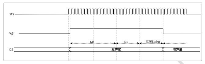
Figure 29-18 I2S MSB justified standard (24-bit frame, CPOL = 0)
