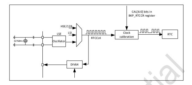
Figure 26-4 RTC calibration chart
