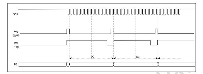
Figure 29-29 I2S PCM standard (16-bit frame, CPOL = 1)
