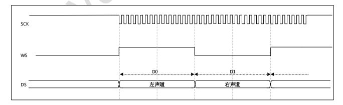
Figure 29-17 I2S MSB justified standard (16/32 bit full accuracy, CPOL = 1)
