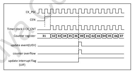
Figure 19-4 Counter timing diagram, internal clock divided by 1
