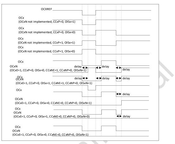
Figure 18-38 Output behavior in response to a break
