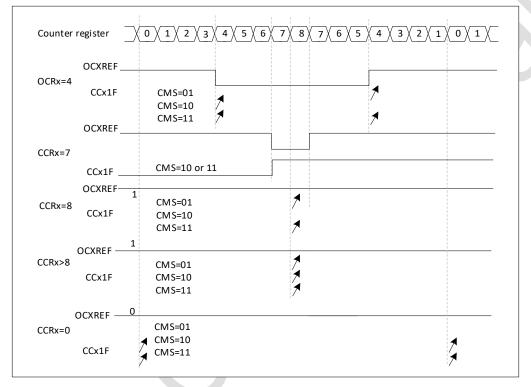
Figure 18-34 Center-aligned PWM waveforms (ARR=8)
