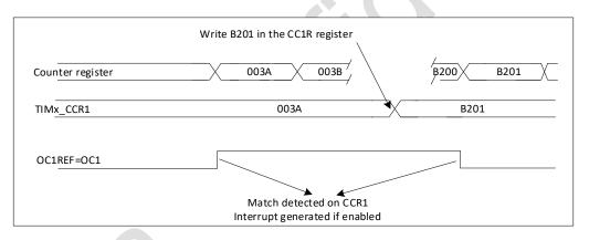
Figure 18-32 Output compare mode, toggle on OC1
