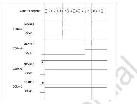
Figure 21-16 Edge-aligned PWM waveform (ARR = 8)
