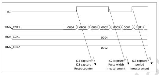
Figure 18-31 PWM input mode timing
