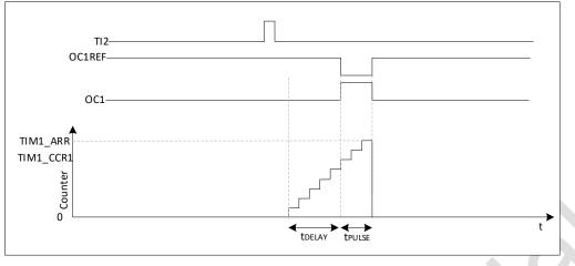
Figure 18-41 Example of one pulse mode
