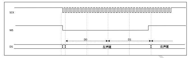
Figure 29-12 I2S Philips protocol (16/32 bit full accuracy, CPOL = 1)
