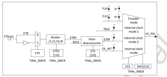
Figure 18-25 TI2 external trigger input block
