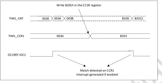
Figure 21-15 Output compare mode, toggle on OC1
