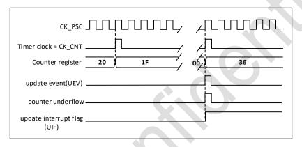
Figure 19-13 Counter timing diagram, internal clock divided by N
