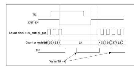
Figure 18-47 Control circuit in Gated mode
