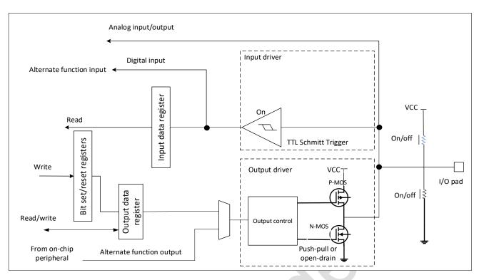
Figure 9-4 Alternate function configuration
