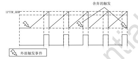
Figure 23-3 Low power timer output waveform, continuous counting mode
