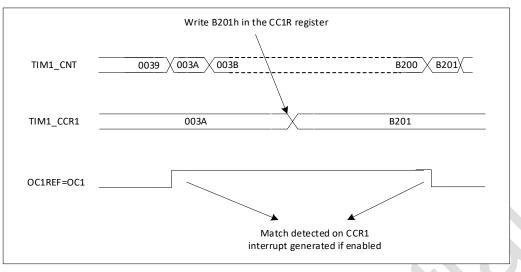
Figure 20-12 Output compare mode, toggle on OC1
