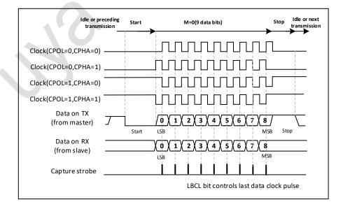
Figure 28-11 USART data clock timing diagram (M=1)
