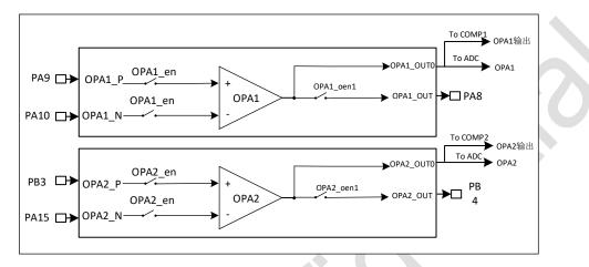
Figure 16-1 OPA architecture block diagram
