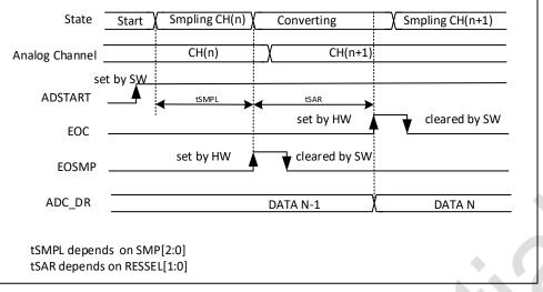
Figure 14-5 Analog-to-digital conversion timing
