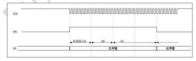
Figure 29-21 I2S MSB justified standard (16-bit extended 32-bit, CPOL = 1)
