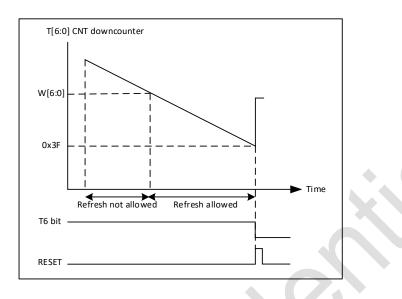
Figure 25-2 Window watchdog timing diagram
