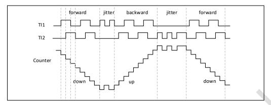
Figure19-35 TI1P1 inverted encoder interface mode example
