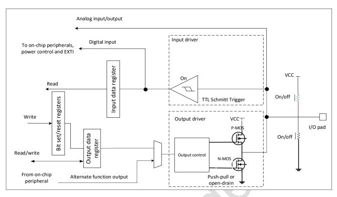
Figure 9-3 Output configuration
