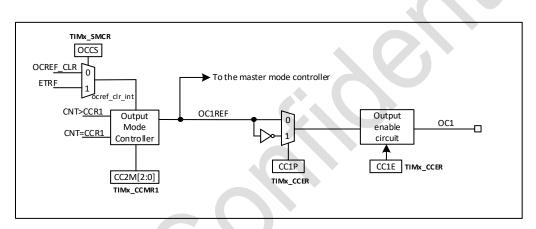
Figure 19-28 Capture/Compare the output portion of the channel (channel 1)
