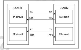
Figure 28-14 Hardware flow control between two USARTs
