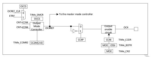
Figure 18-30 Output stage of capture/compare channel (channel 4)
