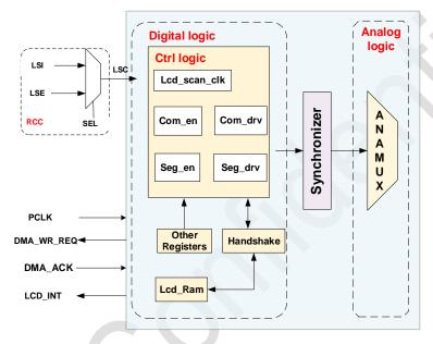
Figure 17-1 LCD control block diagram
