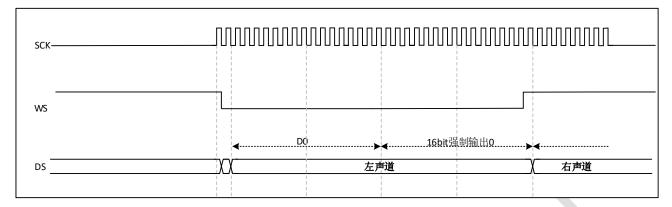
Figure 29-15 I2S Philips protocol (16-bit extended to 32-bit)
