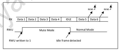
Figure 28-7 Mute mode using Idle line detection
