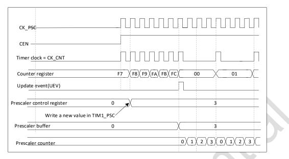
Figure 21-3 Counter timing diagram with prescaler division change from 1 to 4
