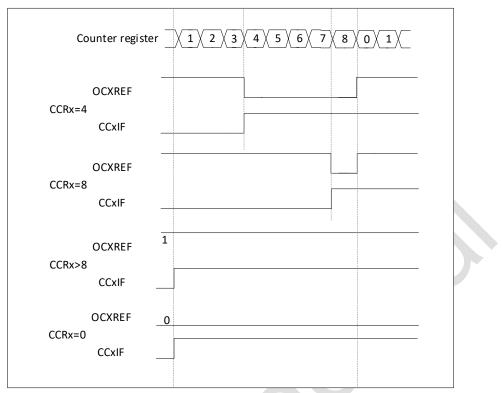
Figure 20-13 Edge-aligned PWM waveforms (ARR=8)
