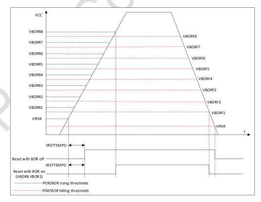
Figure 5-2 POR/PDR/BOR thresholds
