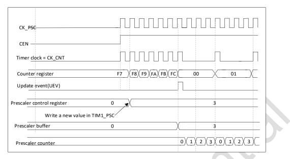
Figure 20-3 Counter timing diagram with prescaler division change from 1 to 4
