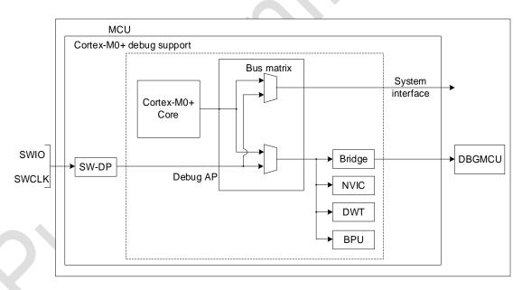
Figure 32-1 DBG block diagram
