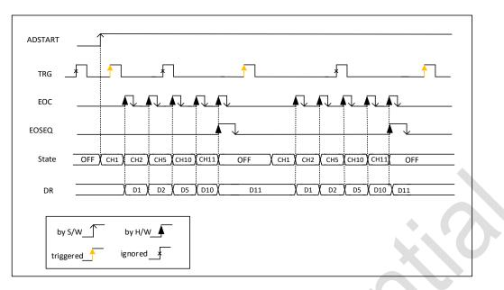
Figure 14-9 Single conversions of a sequence, hardware trigger
