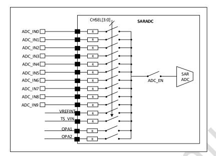
Figure 14-2 ADC channel with analog switch
