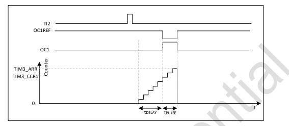
Figure 19-33 Example of one pulse mode
