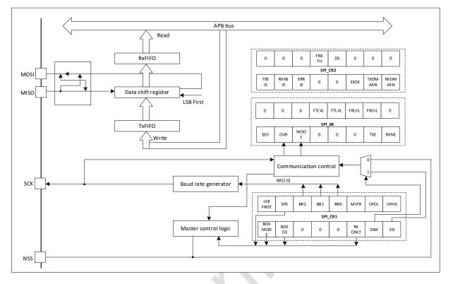
Figure 29-1 SPI block diagram
