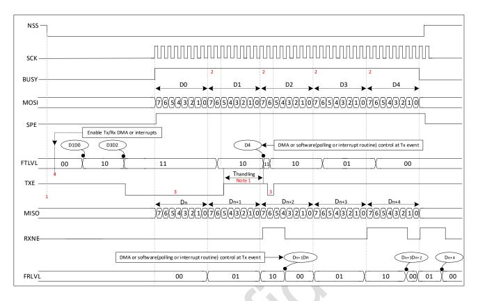
Figure 29-9 Master full-duplex communication (bit frame=8)
