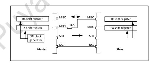
Figure 29-3 Half-duplex single master/ single slave application
