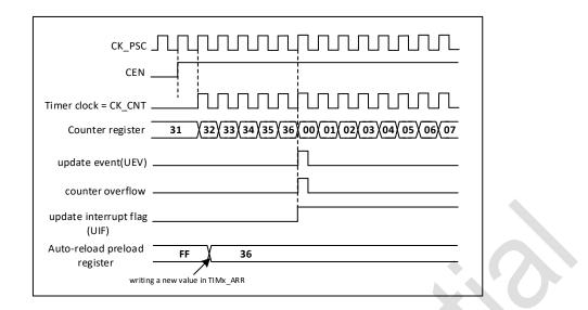
Figure 19-8 counter timing diagram, update event when ARPE = 0 (TIMx \_ ARR is not pre-loaded)
