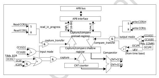
Figure 18-28 Capture/compare channel 1 main circuit
