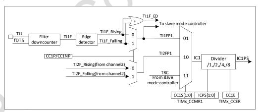
Figure 21-12 Capture/compare channel (example: channel 1 input stage)
