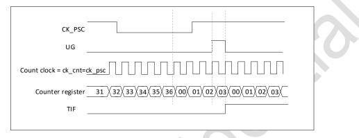
Figure 18-46 Control circuit in reset mode
