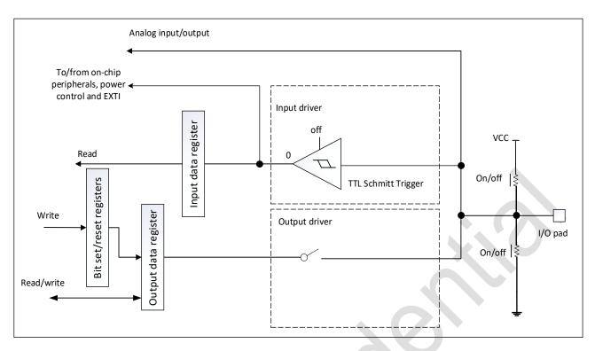
Figure 9-5 High impedance-analog configuration
