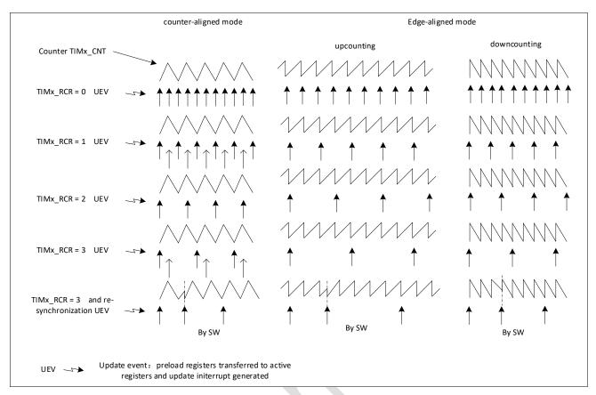
Figure 18-21 Update rate examples depending on mode and TIM1\_RCR register settings
