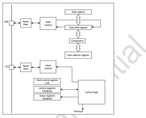
Figure 27-1 I<sup>2</sup>C block diagram
