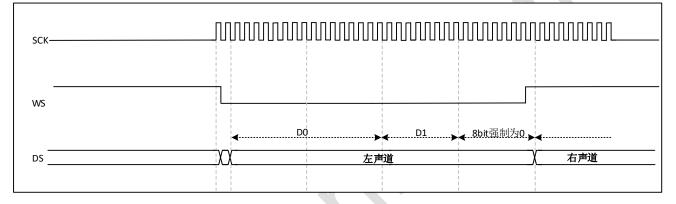
Figure 29-13 I2S Philips protocol (24-bit frame, CPOL = 0)
