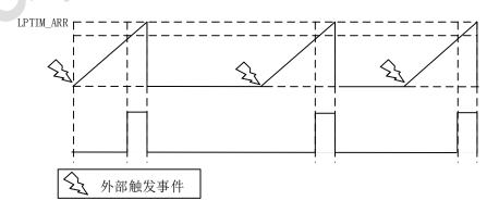
Figure 23-2 Low power timer output waveform, single count mode
