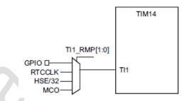
Figure 8-2 Frequency measurement vs. TIM14 capture mode
