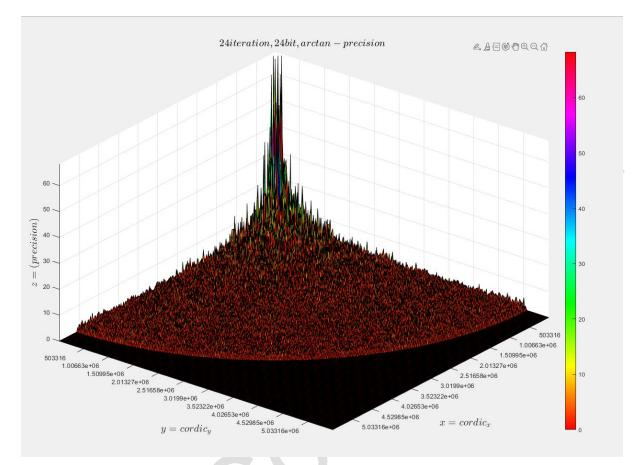
data as x and y axes, and arctan result error as z axis.
