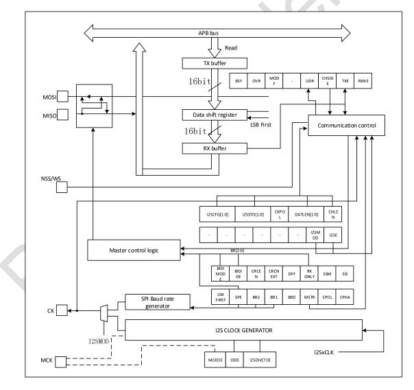
Figure 29-10 I2S block diagram
