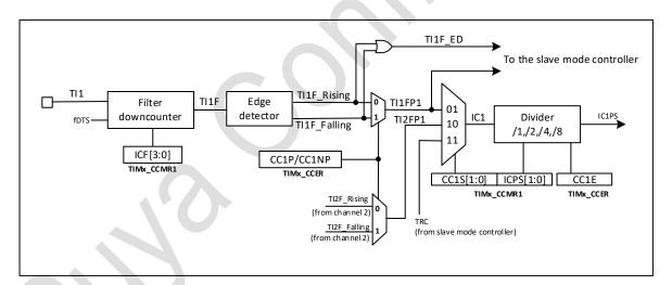
Figure 19-26 Capture/compare channel (example: channel 1 input stage)
