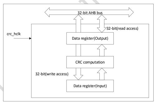
Figure 13-1 CRC calculation unit block diagram
