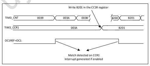
Figure 19-30 Output compare mode, toggle on OC1
