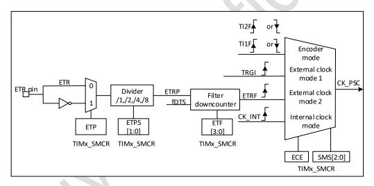
Figure 19-24 ETR External Clock Connection Example
