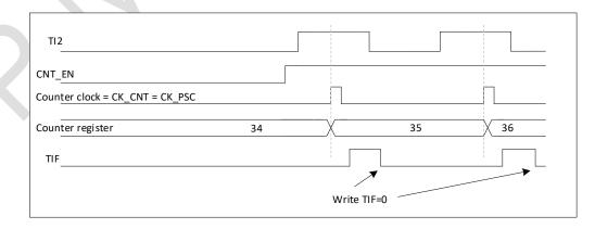
Figure 18-24 Control circuit in external clock mode 1
