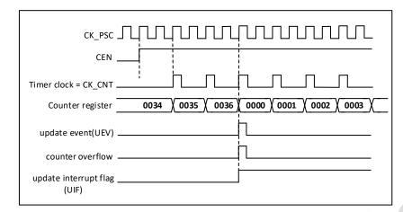
Figure 19-5 Counter timing diagram, internal clock divided by 2
