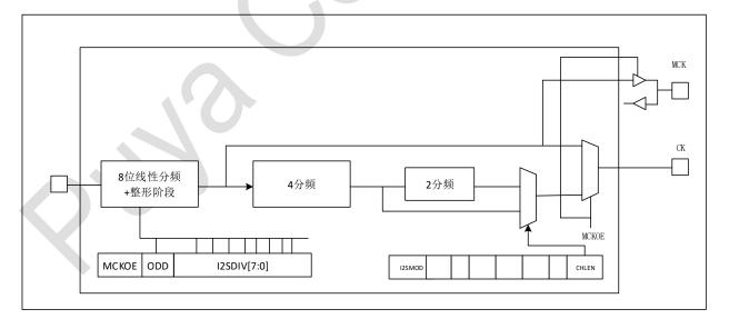
The sampling frequency of the audio may be 96 kHz, 48 kHz, 44.1 kHz, 32 kHz, 22.05 kHz, 16 kHz, 11.025 kHz, or 8 kHz (or any value within this range). In order to obtain the required frequency, it is obtained by setting the linear frequency divider according to the following formula, when the master clock needs to be generated (the MCKOE bit of the register SPI \_ I2SPR is' 1 '): When the frame length of the channel is 16 bits, Fs = I2SxCLK/[(16 \* 2) \* ((2 \* I2SDIV) + ODD) \* 8]
